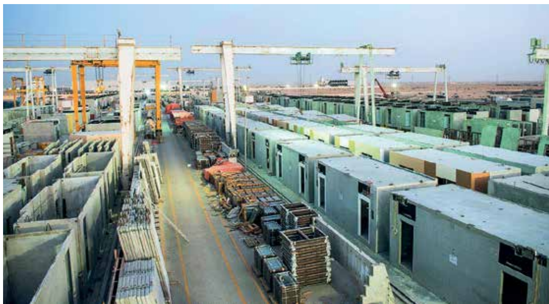
An assembly line of modular housing at a manufacturing site owned by Dubox
